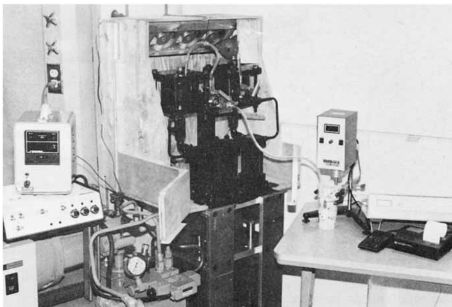
Fig. 2. Photograph of the lab-scale RIM machine.
